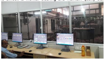
parameters such concentration of cleaning agents and temperature of water to be used for rinsing are stored in the system with no room for error. In totality complete system offers qualitative & financial benefits and apart from this increased working efficiency, saving in energy, water and recovery of cleaning solutions.
